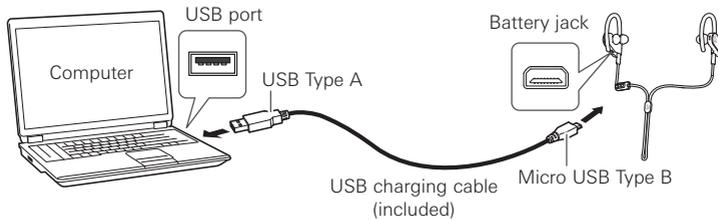
2. Connect the included USB charging cable (USB Type A side) to the computer to start charging.
