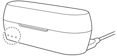
4. When charging is complete, disconnect the USB charging cable (USB Type-A side) from the computer.
